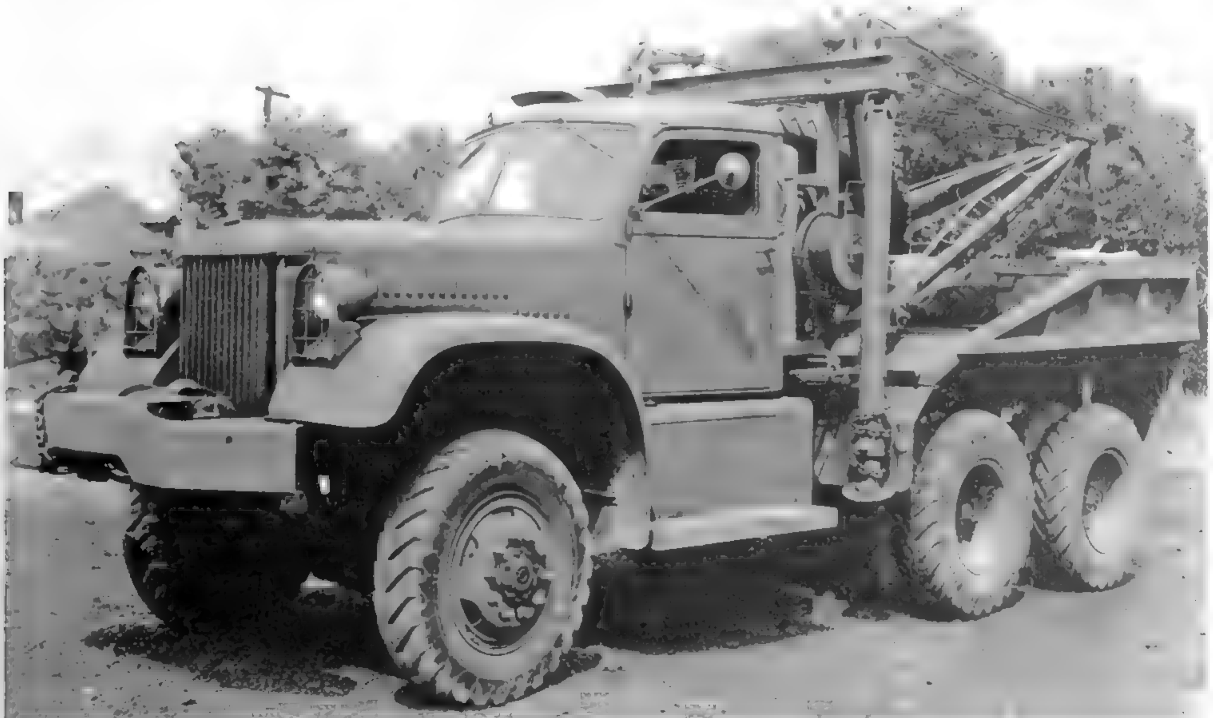
This photograph, taken three days after the attack on Pearl Harbor, illustrates the classic lines of the early Diamond T 969 series wreckers. (Signal Corps photograph from the collection of Bryce Sunderlin)
